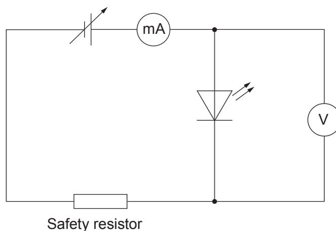
Aled decides that the LED is switched on when a current of 10.0 mA passes through it. He adjusts the variable power supply and records the switching-on pd. He repeats this procedure for different LEDs which emit light of different wavelengths. His results are tabulated below.
