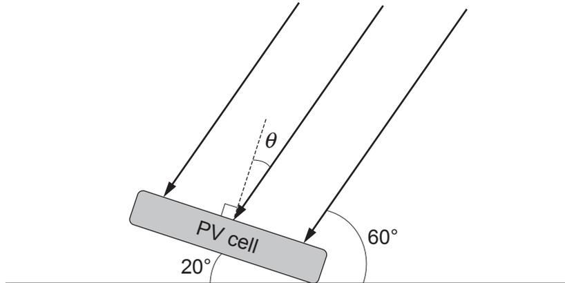
A factory decides to install rooftop PV cells at an angle of 20° to the horizontal. At midday when the Sun's elevation is 60° the solar radiation incident upon the surface of the Earth has an intensity of 600 W m<sup>-2</sup>. An individual PV cell has a conversion efficiency of 20% and is found to produce a power output of 150 W.
