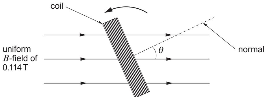
The flux **linkage** of the coil for the angles  $\theta = -5^\circ$  and  $\theta = +5^\circ$  is 1.29 Wb turn in each case.
